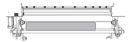
9. Fit the paper tube (core) of the media onto the end cap of the left media holder.
