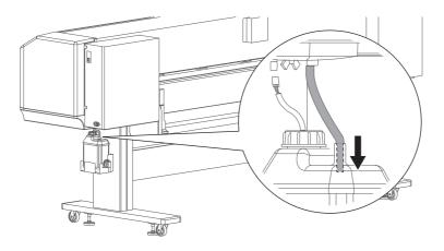
[3] Connect the waste ink sensor cable to the waste ink sensor connector.
