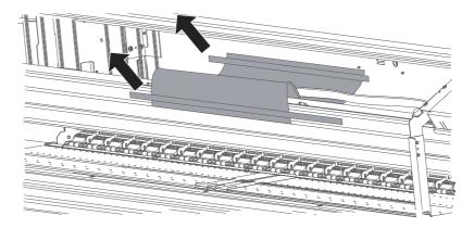
[7] Remove the tape, and move the edge holders to the left and the right edge.
