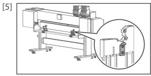
(When looking from the rear side of the printer) Use the screwdriver to loosen two screws securing the roller shaft guide plate to the right media holder.
