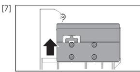
Do the same for the left media holder to slide up the roller shaft guide plate as far as it will go and tighten the screws.
