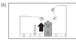
Slide up the roller shaft guide plate as far as it will go and tighten the screws.
