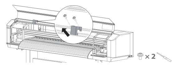
[5] Open the front cover. Remove the wing bolt to remove the shipping bracket from the carriage.
