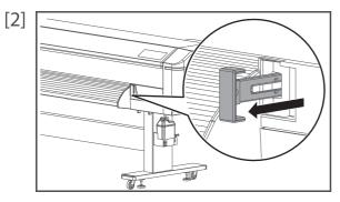
From the front side of the printer, fully pull the media feed lever towards you to release the pressure rollers.
