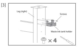
Use the round head screws (×4) to attach the waste ink tank holder to the right leg.
