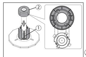
(If you are using 2-inch core roll media), remove the 3-inch adapter from the media flange.
