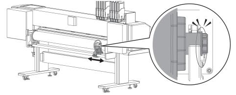
Twist the knob bolt on the right side of the media holder clockwise to tighten.
