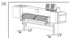
From the rear side of the printer, insert the front edge of the media into the media slot.
