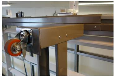
If required, the leg section can be easily removed from the flat bed while still in a vertical position. 2 bolts are holding each leg to the main support frame.
