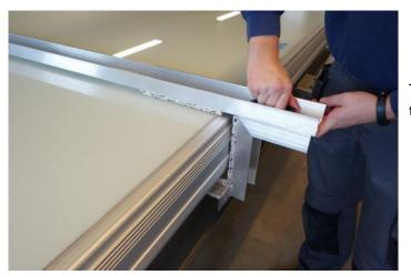
Tighten the locking mechanism on the top of the supports.
