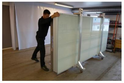
Once in the vertical position, the table can be moved carefully to the final destination.
