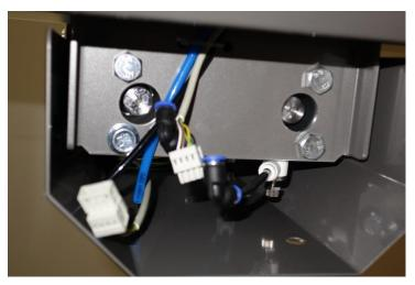
Loosen the quick connectors for the power and the compressed air as showed on the picture.
