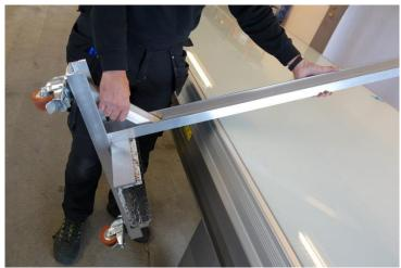
Place the two supports carefully on top of the flatbed as shown in the picture.
