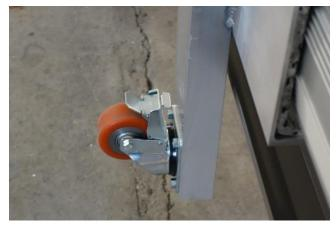
*Important!* Turn the castors of the device as shown on the picture and *lock*.
