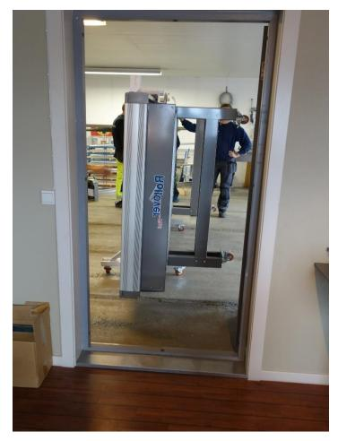
The device enables passing through a standard door – if needed the castors can be temporarely removed.
