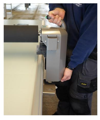
The roller gantry can now be carefully lifted off the flatbed and placed on the floor. *Attention!* This opeation requires 1 person on each side of the flatbed.
