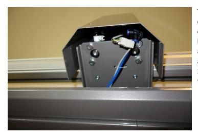
To enable the use of the transport device, the roller gantry must be lifted off the table. Underneath each housing, you will find the 4 bolts attaching them to the wire brackets, and also the quick connectors for the 24V power and the compressed air tubes (black and blue).
