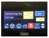
This screen is used to purge and clean the system.
