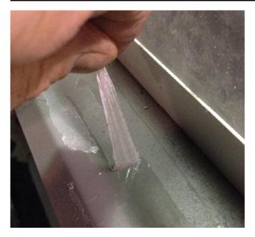
This photo shows dried pre-treat solution being peeled up from the inside of the spray chamber. It is important to clean your unit to protect your investment.
