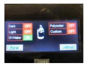
Make sure you select the di water (same as distilled water) when purging the unit.
