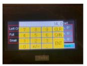
This photo shows the basic entry screen - in this example for numeric input. You must press "ENT" to save the input you selected.
