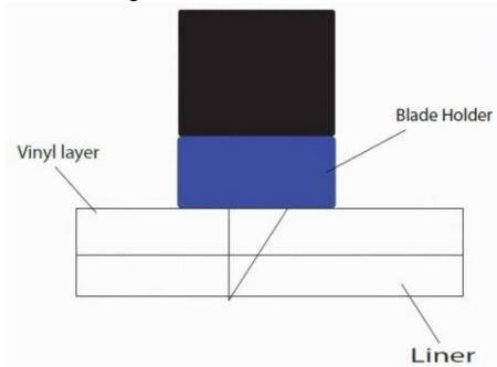
Note: Blade length should cover overall thickness of media.
